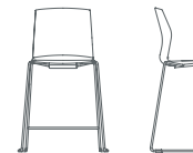
960-CH24-NA Celebrate Counter height stool H38.75 W21 D20.5 SEAT H24 W17 D17.75
